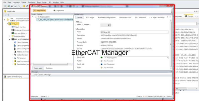
2. Click on the slave in the *SPEED7 EtherCAT Manager* and select the 'PDO assign' tab in the 'Device editor'.
