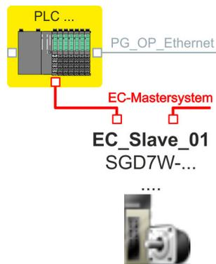
⇒ The *Sigma-7W* double-axis drive is connected to your EC master system.
