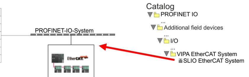
1. Navigate in the hardware catalog to the directory 'PROFINET IO' → 'Additional field devices' → 'I/O' → 'VIPA EtherCAT System' and connect the IO device 'SLIO EtherCAT System' to your PROFINET system.
