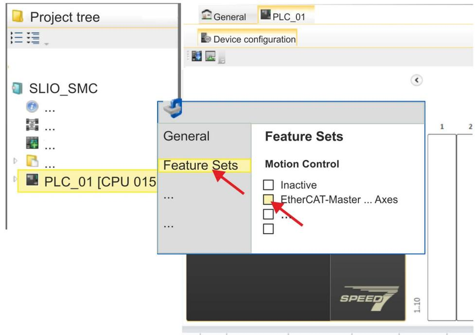
2. Click at 'Feature Sets' and activate at 'Motion Control' the parameter 'EtherCAT-Master... Axes'. The number of axes is not relevant in this example.
