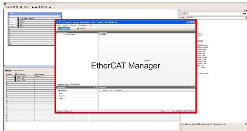
3. ➤ For the *Sigma-7S* EtherCAT drive to be configured in the *SPEED7 EtherCAT Manager*, the corresponding ESI file must be installed. The ESI file for the *Sigma-7S* EtherCAT drive can be found under [www.yaskawa.eu.com](http://www.yaskawa.eu.com) at 'Service ➔ Drives & Motion Software'. Download the according ESI file for your drive. Unzip this if necessary.
