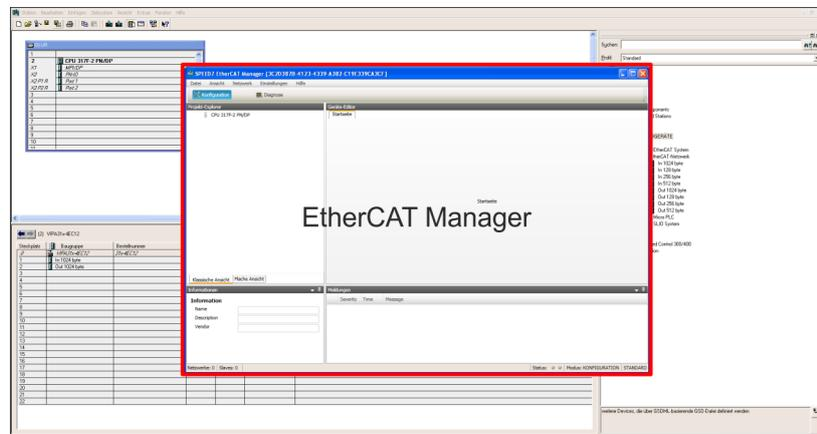
3. ➤ For the *Sigma-7W* EtherCAT drive to be configured in the *SPEED7 EtherCAT Manager*, the corresponding ESI file must be installed. The ESI file for the *Sigma-7W* EtherCAT double-axis drive can be found under [www.yaskawa.eu.com](http://www.yaskawa.eu.com) at 'Service ➔ Drives & Motion Software'. Download the according ESI file for your drive. Unzip this if necessary.
