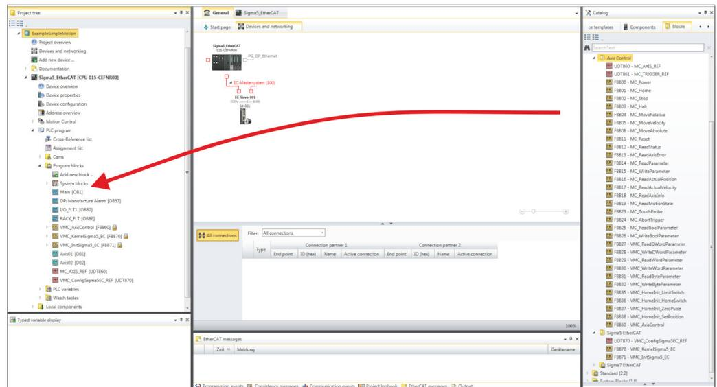
3. In the '*Catalog*', open the '*Simple Motion Control*' library at '*Blocks*' and drag and drop the following blocks into '*Program blocks*' of the *Project tree*:
