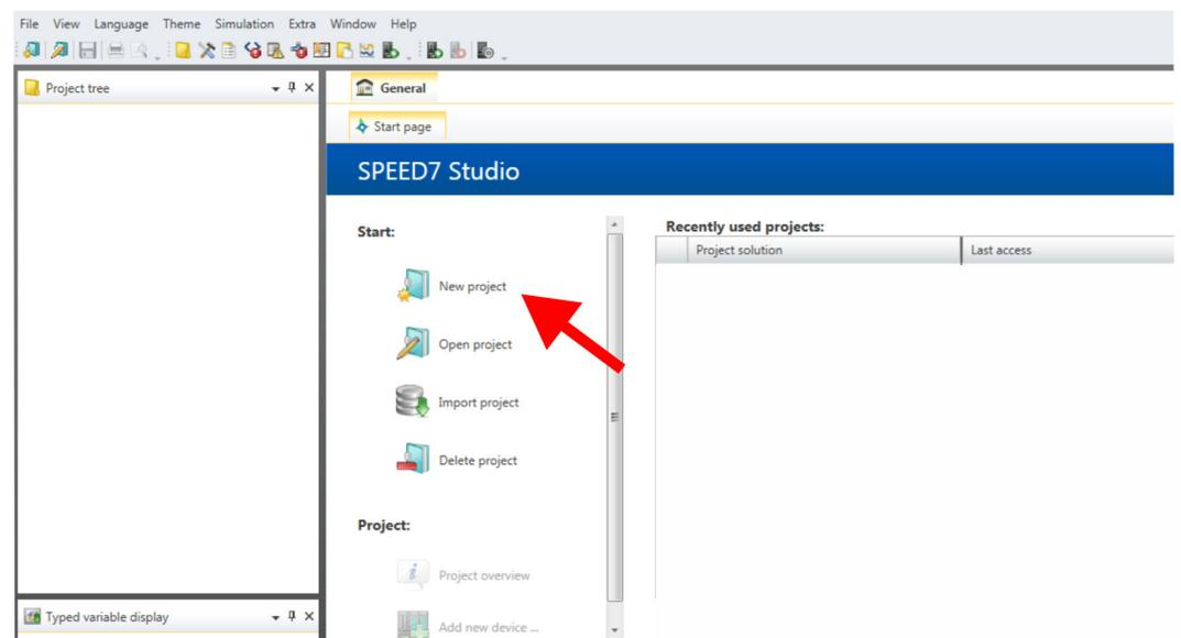
**2.** Create a new project at the start page with '*New project*'.⇒ A new project is created and the view '*Devices and networking*' is shown.
