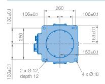
Mounting options: Floor, ceiling, wall, tilt\* IP Protection: IP67
