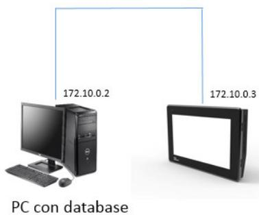
If the CREW application has been developed for a PC based device (Scada) both the Crew runtime and the database can run on the same PC.
