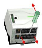
**8.** Remove the connectors, which are not necessary at the CPU.
