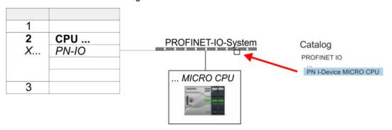
Open the properties dialog of the PROFINET IO controller of the CPU by a double-click at 'PN-IO' and assign a 'Device name' for the I-Device in the Register 'General'.
