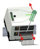
module exchange with a fix wiring. For this each connector has indentations for unlocking at the top. Unlocking takes place by the following proceeding:
