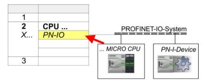
3. For 'PN-IO' at 'slot' 'X...' assign an IP address via the properties dialog.
