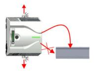
3. Pull the locking levers of the CPU outwards until these engage audible.
