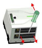
**7.** Remove the connectors, which are not necessary at the CPU.
