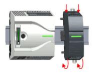
To mount plug the periphery module from the top onto the mounting rail and turn the periphery module downward until it rests on the mounting rail.
