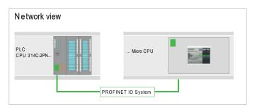
1. After installing the GSDML the 'PN I-Device for ... CPU' can be found in the hardware catalog at 'Other field devices → PROFINET IO → I/O → VIPA ...
