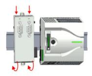
To mount plug the extension module from the top onto the mounting rail and turn the extension module downward until it rests on the mounting rail.
