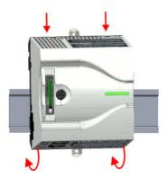
Plug the CPU from the top onto the mounting rail and turn the CPU downward until it rests on the mounting rail.
