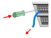
The wire is to be removed by means of a screwdriver with 2.5mm blade width.
