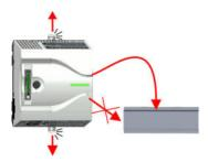
**2.** The CPU has a locking lever on the upper and lower side. Pull these levers outwards as shown in the figure, until these engage audible.
