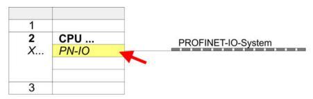
The PROFINET interface of the PROFINET IO controller is parametrized with PN-IO, the port with Port 1. In the following these parameters for PN-IO and Port 1 are described.
