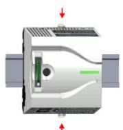
**6.** To fix the CPU at the mounting rail, move the locking levers back to the initial position.
