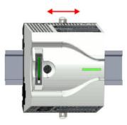
**5.** Move the CPU on the mounting rail at its position.
