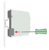
**2.** The extension module has a locking lever on the upper and lower side. Pull these levers outwards as shown in the figure, until these engage audible.
