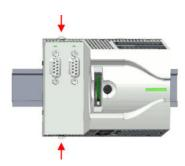
**5.** To fix the extension module at the mounting rail, move the locking levers back to the initial position.
