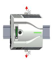
**2.** Remove the CPU with a rotation upwards from the mounting rail.
