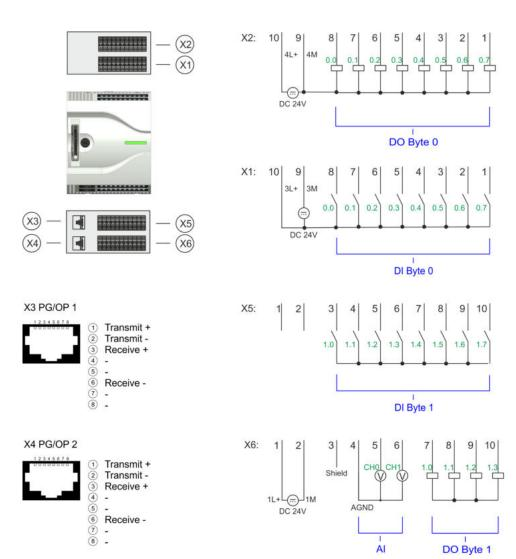
Wiring > Wiring CPU
