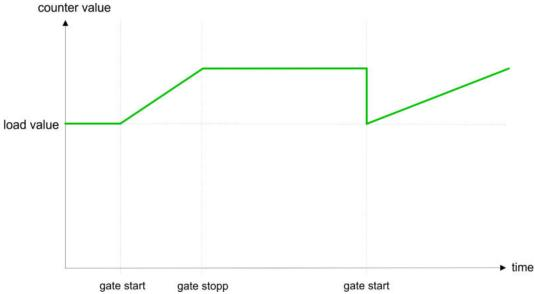
At *interrupt function*, the counter starts counting with the last recent counter value after gate restart.
