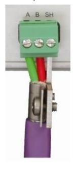
It is recommended to use the supplied ground clip to attach the cable shield to the screw connector, for easier shield connection and better strain relief.
