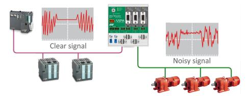
Because of the isolation and intelligence the PROFIBUS MultiRepeater provides, it can be used as a barrier for electrically sensitive segments. This keeps the backbone and other Channels clean.
