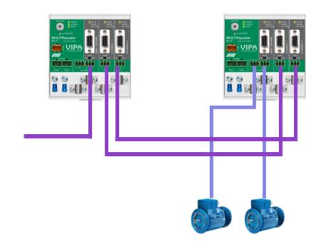
The telegrams are transferred onto both redundant channels. The logic inside the Repeater determines which telegram is used to be transferred onto the other channels. A message received by a redundant channel is repeated on all other channels, except the other redundant channel. A message received by a normal channel is repeated on all other channels.
