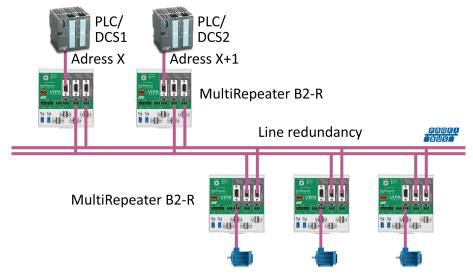
If bus redundancy is enabled, 2 segments will form a redundant pair. Short circuit protection on each spur line is automatically provided.
