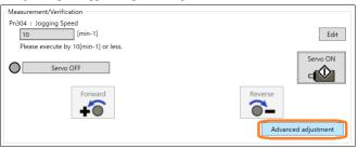
We recommend setting the speed ripple compensation gain to 100% or less because speed ripple may grow larger if the gain setting is too high.
