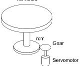
Because the turntable moves in only one direction, the upper limit to the number of rotations that can be counted by an absolute encoder will eventually be exceeded.
