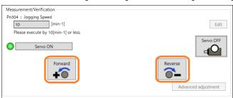
The servomotor shaft will rotate at the preset jogging speed while you hold down the [Forward] or [Reverse] button and the speed ripple will be measured.
