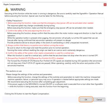
A jogging speed for the speed ripple measurement will be automatically set.
