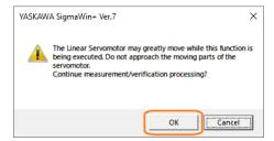
The linear servomotor will move to the end point that was set and speed ripple will be measured.
