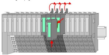
**2.** Press the unlocking lever at the lower side of the just mounted right module of the module group and pull it forward.
