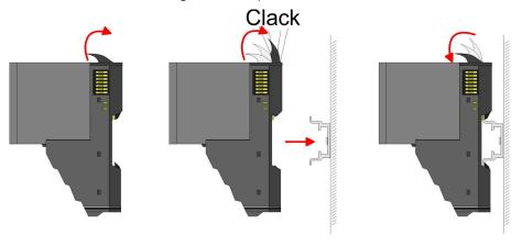
For the exchange of a electronic module, the electronic module may be pulled forward after pressing the unlocking lever at the lower side of the module. For installation plug the electronic module guided by the strips at the lower side until this engages audible to the terminal module.
