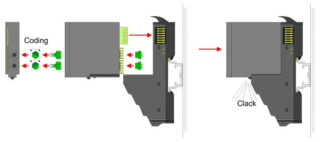
Each electronic module has on its back 2 coding sockets for coding jacks. Due to the characteristics, with the coding jack 6 different positions can be plugged, each. Thus there are 36 possible combinations for coding with the use of both coding sockets.
