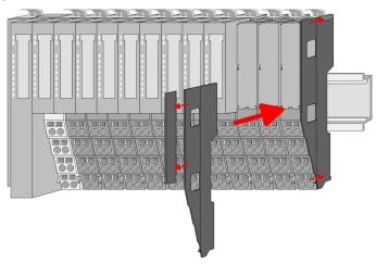
If the last module is a clamp module, for adaptation the upper part of the bus cover is to be removed
