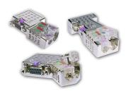
In PROFIBUS all participants are wired parallel. For that purpose, the bus cable must be feed-through. Via the order number 972-0DP10 you may order the bus connector "EasyConn". This is a bus connector with switchable terminating resistor and integrated bus diagnostic.
