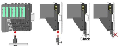
The shield bus carrier (available as accessory) serves to carry the shield bus to connect cable shields. The shield bus carrier is mounted underneath the terminal of the terminal module. With a flat mounting rail for adaption to a flat mounting rail you may remove the spacer of the shield bus carrier.
