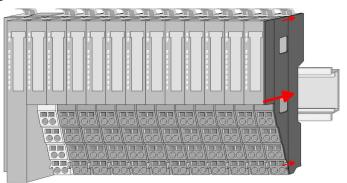
After mounting the whole system, to protect the backplane bus connectors at the last module you have to mount the bus cover, now.
