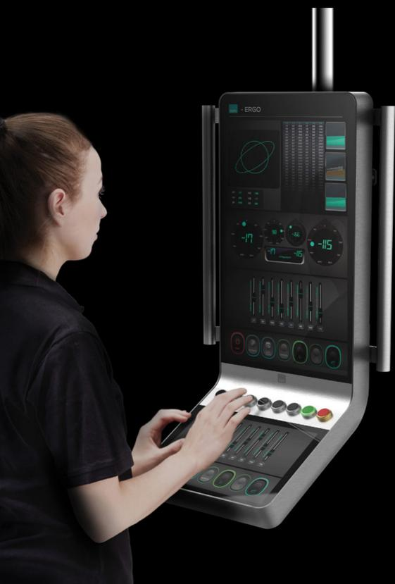
Thanks to its unique level of control and configurability, ERGO perfectly embodies the new concept of human-machine interface 4.0. This device features a flat projected capacitive multi-touch screen and a 21.5" million colors TFT display, and offers users the possibility to choose among numerous configuration options, which include a second 12.1" HMI, touch keypads and additional buttons. Furthermore, ERGO can be supplied with a powerful x86
