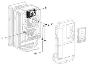
Figure 5 Connect the Ground Wire
