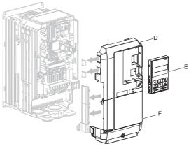
Figure 12 Replace the Front Covers and Digital Operator
