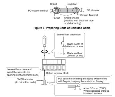
Figure 7 Preparing and Connecting Cable Wiring
