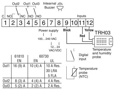
16A max. on the relays common pole (C = terminal 1); 12A max. on model with removable connectors.
