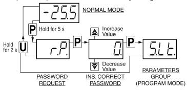
**Notes:** 1. All parameters are configured by default as "protected by password" so that by simply setting the £PP parameter they are all password protected.
