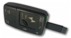
This device it is mainly usable for serial programming those instruments that need the same parameters configuration or to keep a copy of the parameters setting of an instrument and allow its fast duplication.
