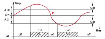
The maximum and minimum temperature alarms can be disabled setting RHE and RLE = oF.
