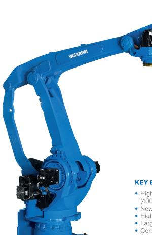
With over 1700 cycles per hour, the fast and powerful 4-axis MOTOMAN PL190 robot offers top performance for box, carton and bag palletizing for end-of-line packaging and logistics applications.
