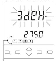
The red led of the activated alarm output is on.
