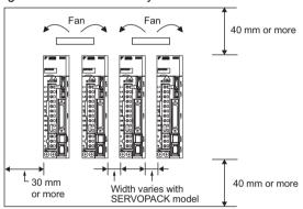
Leave sufficient space on each side and at the top and the bottom of each SERVO-PACK. The width on each side varies in accordance with the models of the SERVO-PACKS used.
