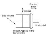
The servomotor will withstand the following vibration acceleration in three directions: vertical, side to side, and front to back.
