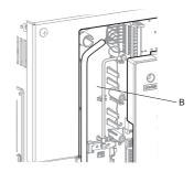
B – Use the open space provided inside the drive to route option card wiring.
