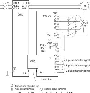
Figure 5 Wiring the Option Card and PG
