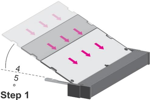
**Step 1:** Insert the memory card into the slot while making sure 1) the notch and the key are aligned, and 2) the non-connector end rises approximately 45 degrees horizontally. Press the card firmly into the socket while applying and maintaining even pressure on both ends.
