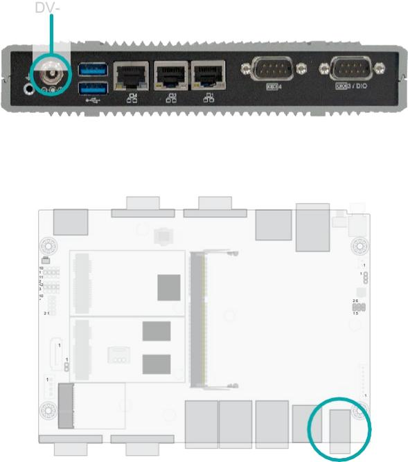
The 9~36V DC-In coaxial supports wide-range voltage power connection.
