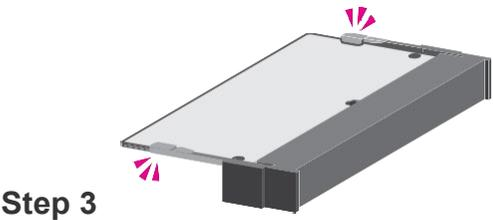
**Step 3:** The clips snap automatically and abruptly to the retention notches of the card sounding a distinctive click, and lock the card in place. Inspect that the clip sits in the notch. If not, please pull the clips outward, release and remove the card, and mount it again.
