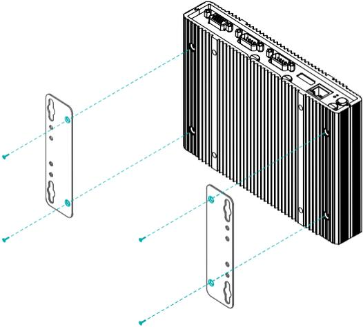
The pre-drilled mounting holes on the brackets allow for different wall mount distances. The assembly can either be screwed right onto a wall or hung on steps screws.
