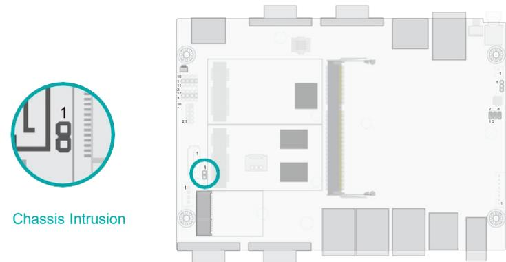
■ Chassis Intrusion Pin Assignment
