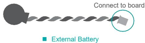
The external lithium ion battery supplies power to the real-time clock and CMOS memory as an auxiliary source of power when the main power is shut off.
