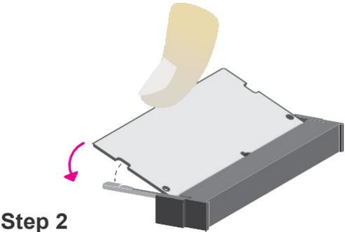
**Step 2:** Press the end of the card far from the socket down while making sure the retention notch and the clip align as indicated by the dot-ted line in the illustration. If the retention notch and the clip do not align, please remove the card and re-insert it. Press the card all the way down.
