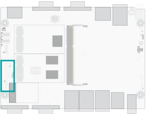
The Serial ATA (SATA) connectors are used to connect the Serial ATA device. SATA 3.0 is supported by the five SATA ports and provides data rate up to 6Gb/s. Connect one end of the Serial ATA cable to a SATA connector and the other end to your Serial ATA device.
