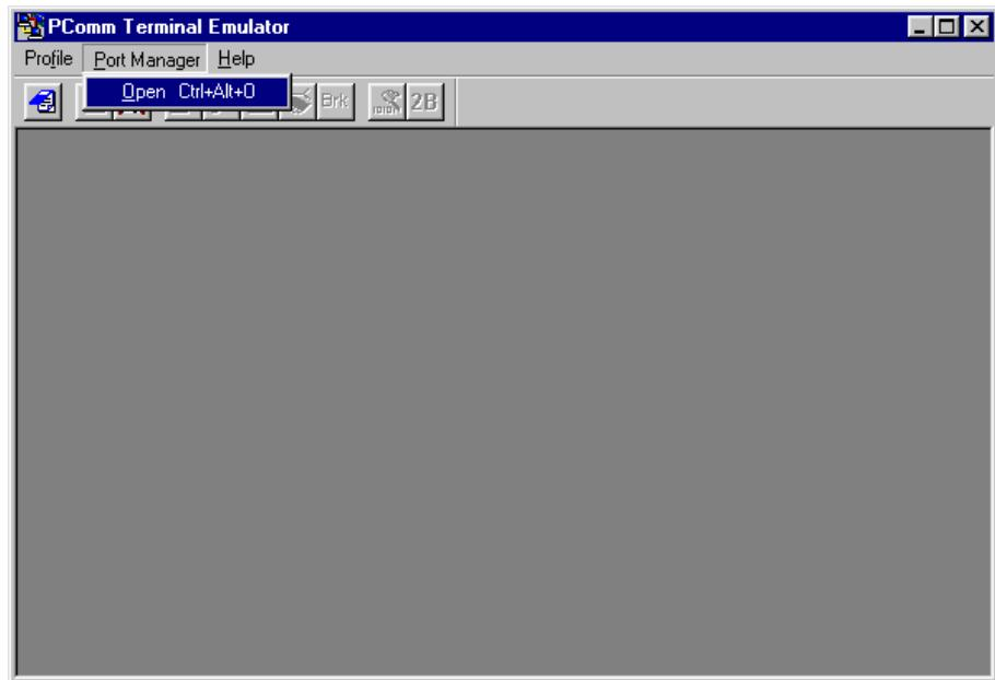
3. The Property window should open. On the **Communication Parameter** tab for **Ports**, select the COM port that is being used for the console connection. Set the other fields as follows:
