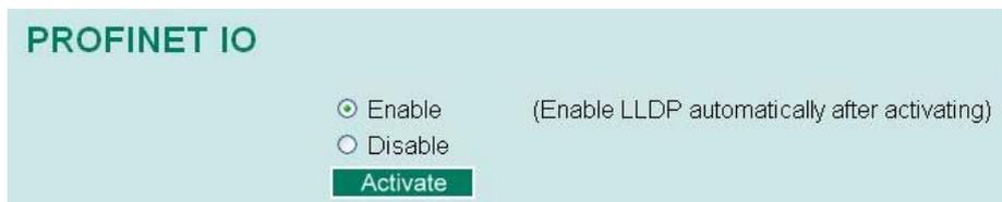
Select the **Enable** option and click [Activate] to enable PROFINET I/O. With PROFINET I/O enabled, PROFINET type LLDP will be enabled automatically. Select the **Disable** option and click [Activate] to disable PROFINET I/O, the switch will disable PROFINET type LLDP and use standard LLDP.
