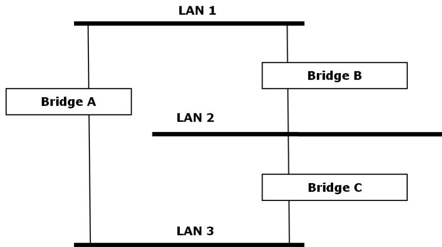
If STP is enabled, it will detect duplicate paths and prevent, or block, one of the paths from forwarding traffic. In the following example, STP determined that traffic from LAN segment 2 to LAN segment 1 should flow through bridges C and A since this path has a greater bandwidth and is therefore more efficient.
