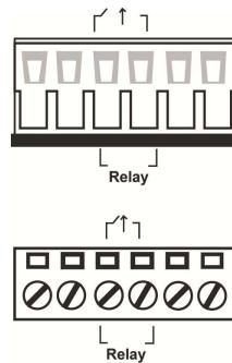
→ **FAULT:** The two middle contacts of the 6-contact terminal block connector are used to detect both power faults and port faults. The two wires attached to the fault contacts form an open circuit when: A relay warning event is triggered.
