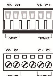
1. → Insert the negative/positive DC wires into the V-/V+ terminals, respectively.
