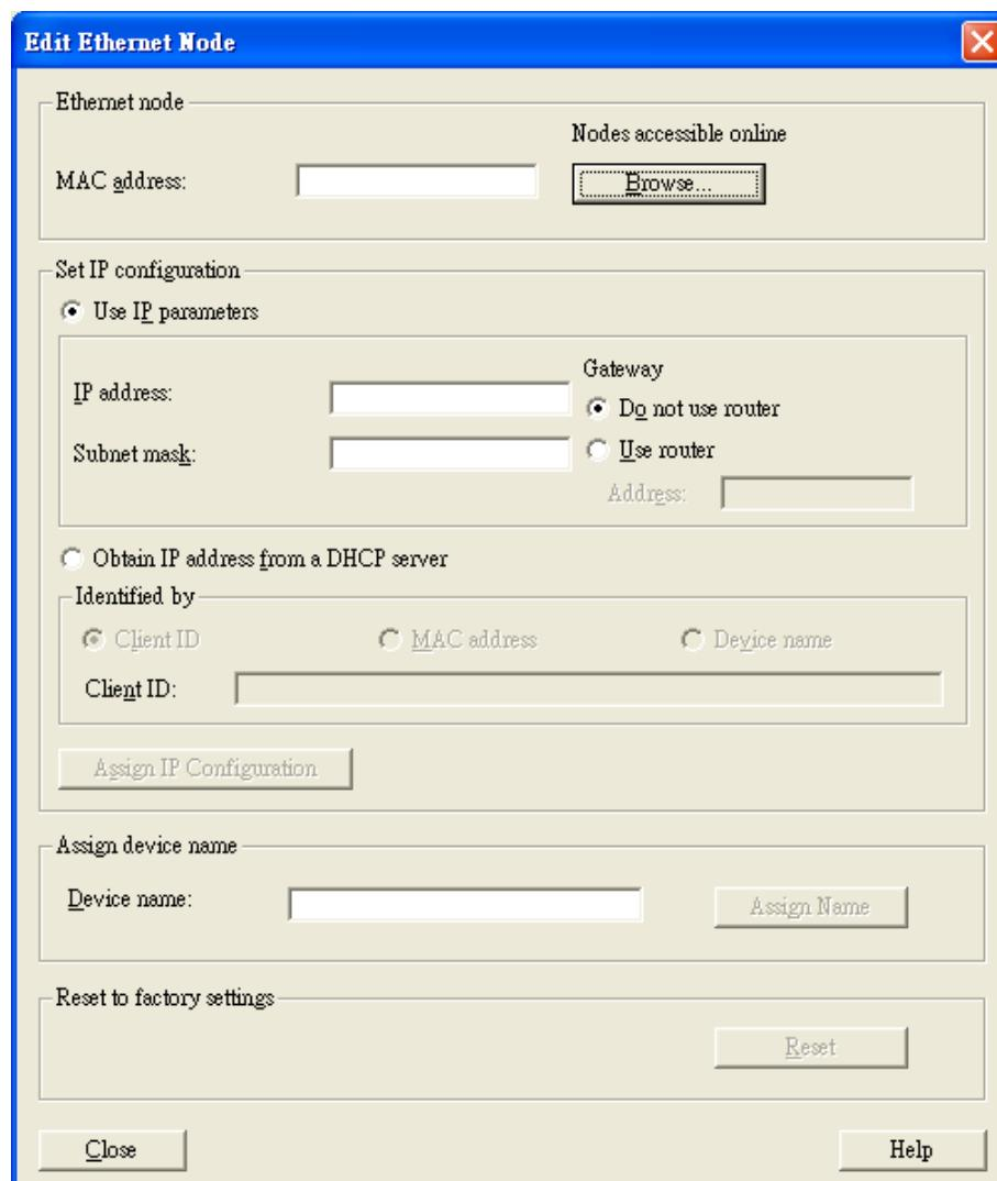
9. ➤ Click [Start] to search devices. Use Siemens STEP®7 through PROFINET DCP to discover devices in networks. Find PLC/switch IP addresses, MAC addresses, and device names here.
