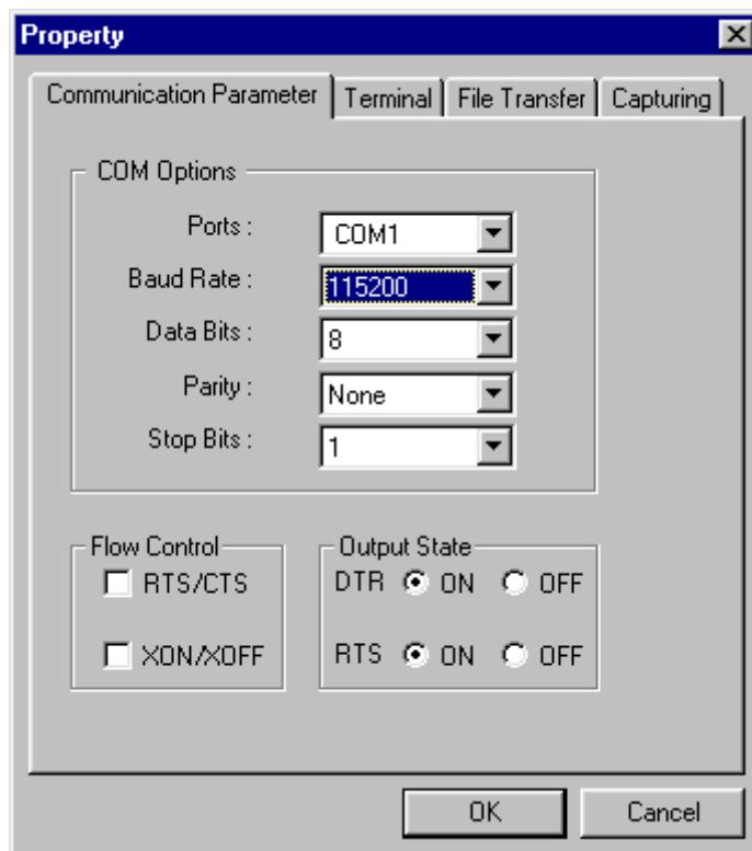
Serial Console Configuration (115200, None, 8, 1, VT100)
