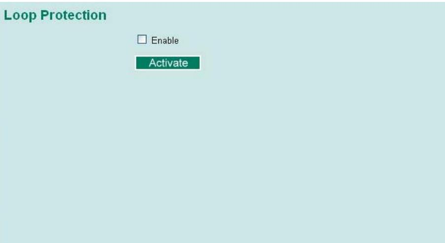
Check the Enable box and click Activate to enable the Loop protection.
