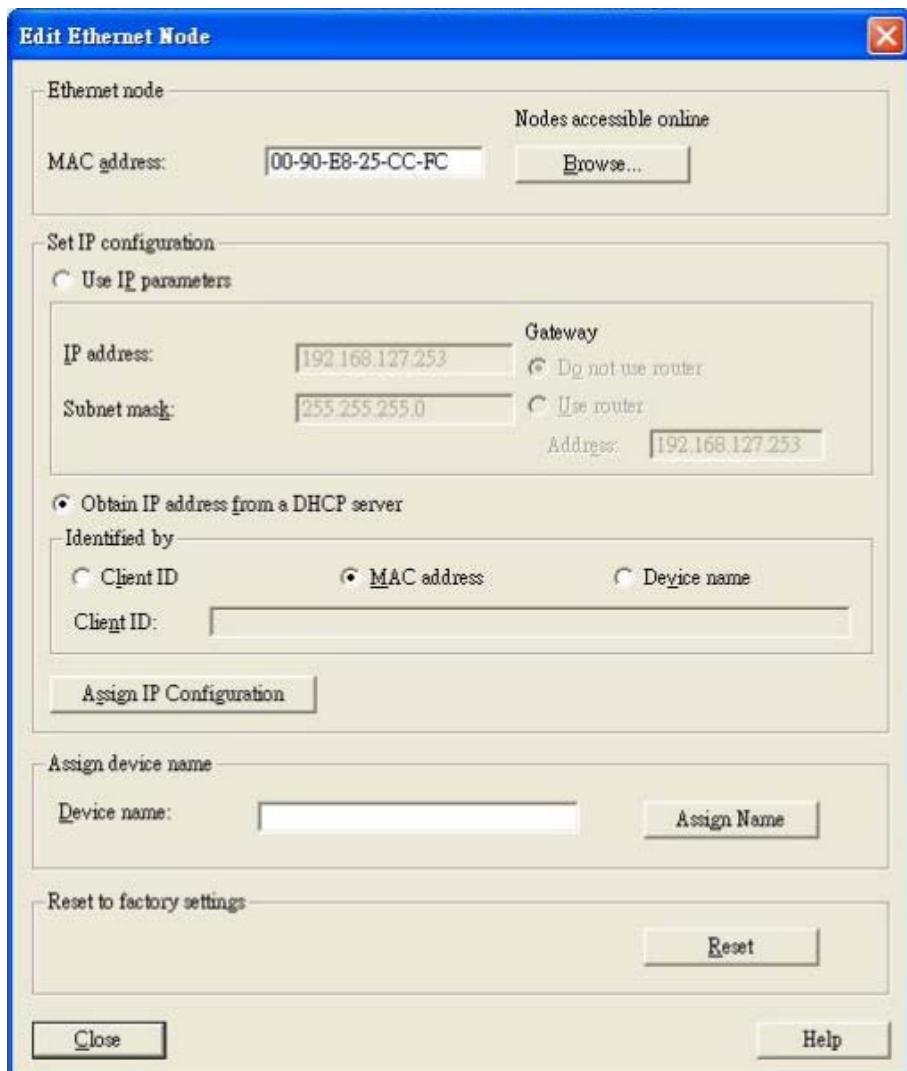
⇒ After the IP has been assigned by DHCP, click [Browse] again to check the assigned IP address.
