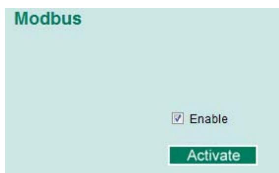
Select the checkbox and click [Activate] to enable the Modbus TCP.
