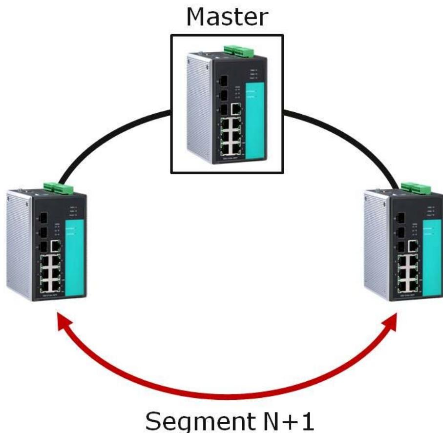
**Determining the Redundant Path of a "Turbo Ring V2" Ring**
