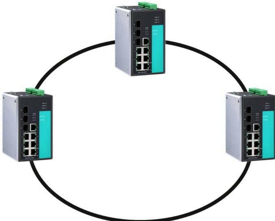
1. Select any two ports as redundant ports.
