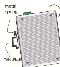
2. The DIN-Rail attachment unit will snap into place as shown.
