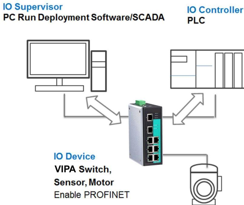
There are 3 major character types defined by PROFINET I/O, including I/O controller, I/O supervisor, and I/O devices. Switches are considered I/O devices.
