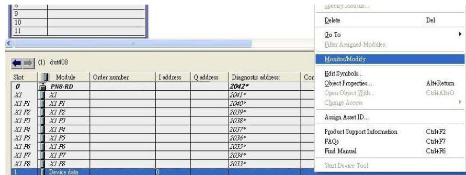
Use Monitor to check the input data value. In this dialog, you can see the status value of each address. Please refer to the **PROFINET Cyclic I/O data table** to see the meaning of each bit. For example, address 0.1 is Bit 1 in the PROFINET Cyclic I/O data table. It represents Power 1 status of the switch. 1 means Power 1 exists and **Green** will be displayed in the **Modify/monitor** window
