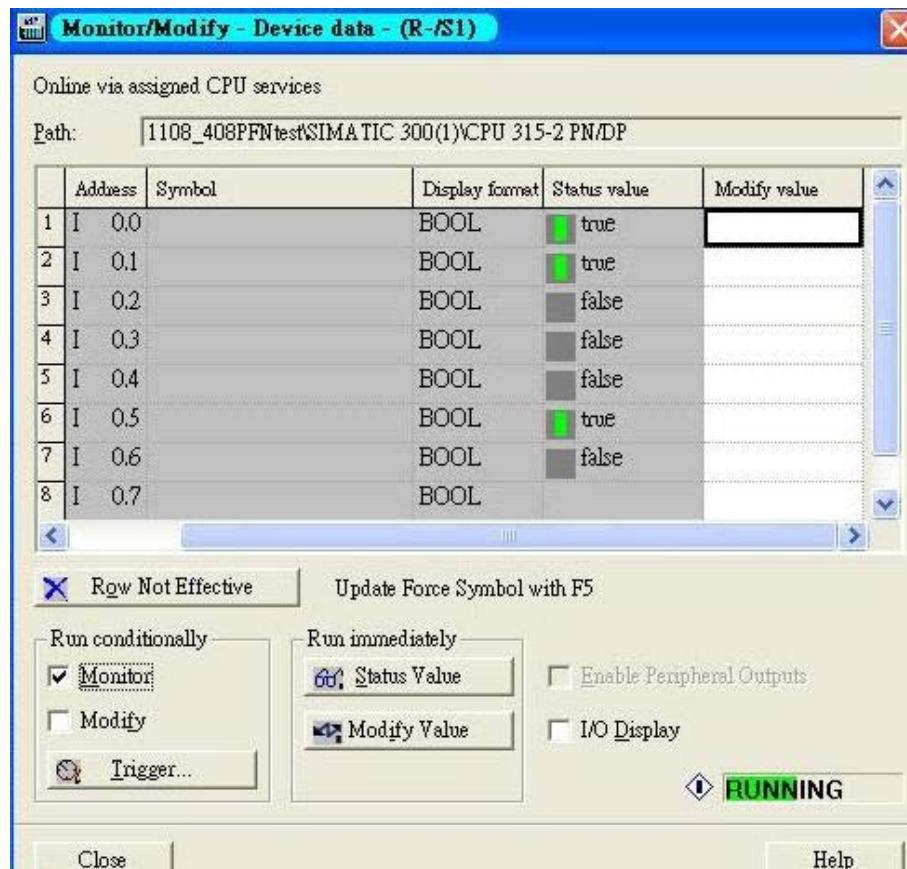
To monitor Port data, follow the same steps, drag **Port data** in the side bar and drop it onto **slot 2**. VIPA PROFINET I/O cyclic data in the slot 1 and 2
