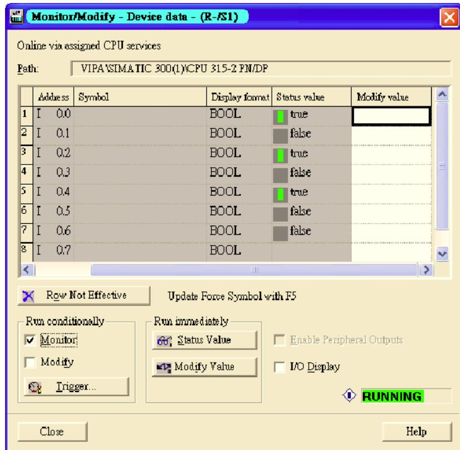
Monitor Port I/O Cyclic Data in Siemens SIMATIC STEP®7
