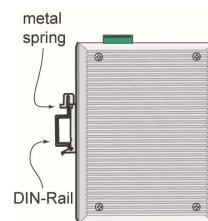
To remove the VIPA Switch from the DIN-Rail, simply reverse Steps 1 and 2.
