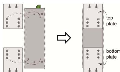
2. ➔ Mounting the Switch on the wall requires 4 screws. Use the switch, with wall mount plates attached, as a guide to mark the correct locations of the 4 screws. The heads of the screws should be less than 6.0 mm in diameter, and the shafts should be less than 3.5 mm in diameter, as shown in the figure at the right.
