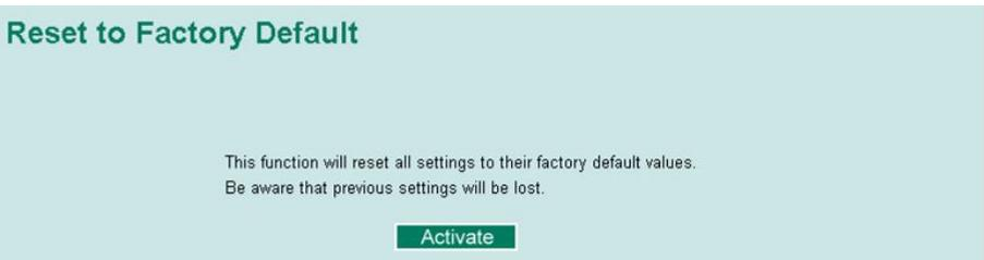
This function provides users with a quick way of restoring the VIPA switch’s configuration to factory defaults. The function is available in the serial, Telnet, and web consoles.
