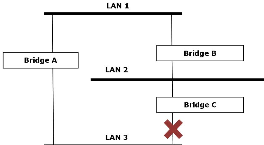
STP will determine which path between each bridged segment is most efficient, and then assign a specific reference point on the network. When the most efficient path has been identified, the other paths are blocked. In the previous 3 figures, STP first determined that the path through bridge C was the most efficient, and as a result, blocked the path through bridge B. After the failure of bridge C, STP re-evaluated the situation and opened the path through Bridge B.
