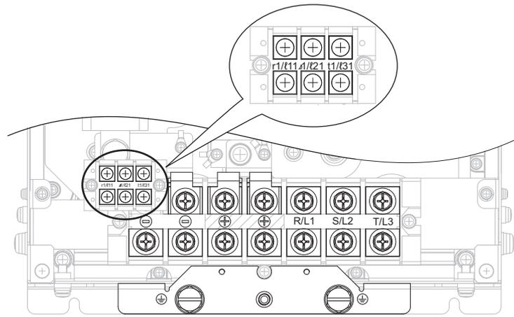
**Figure 3.7 Main Circuit Terminal Block Configuration (Models 4A0053, 4A0073)**
