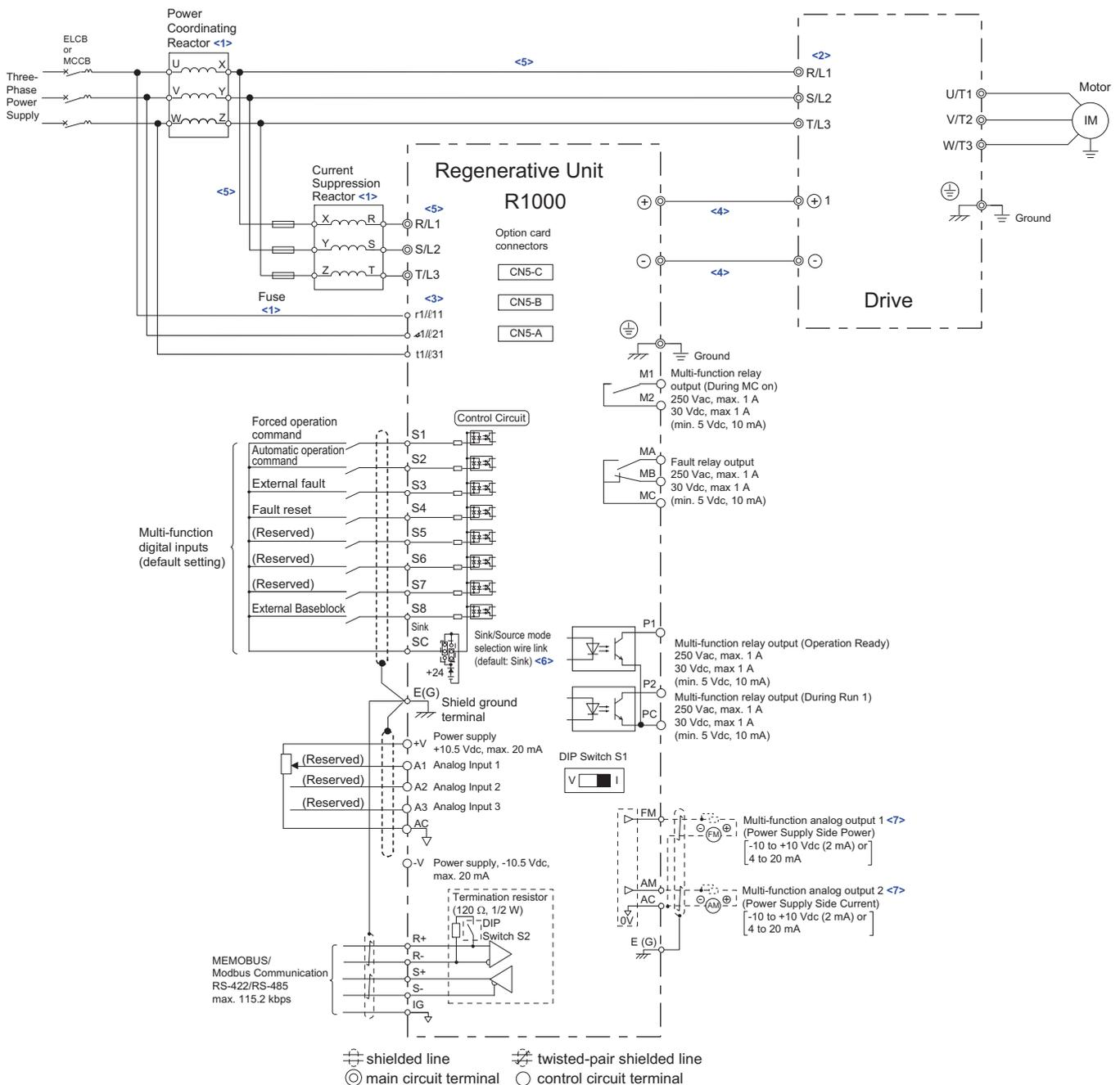
Figure 3.1 Standard Connection Diagram (example: model 2A0007)
