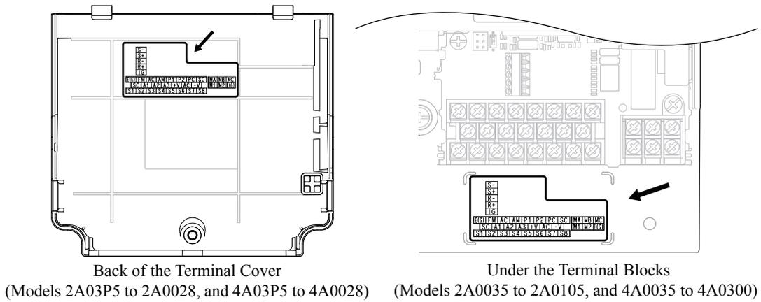
Figure 3.23 Location of Terminal Block Arrangement Diagram
