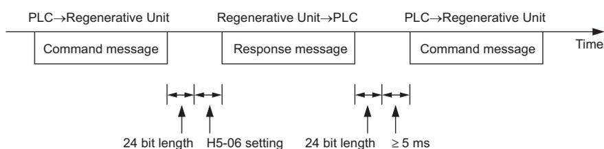
Figure C.4 Regenerative Unit Transmit Wait Time Setting
