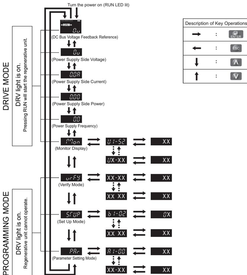
Figure 4.2 Digital Operator Menu and Screen Structure
