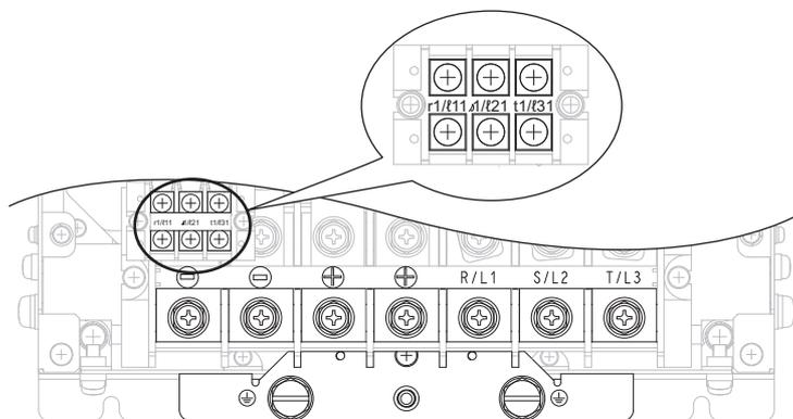
Figure 3.6 Main Circuit Terminal Block Configuration (Models 2A0053)
