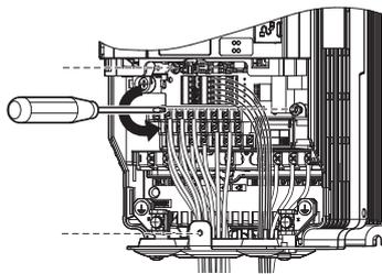
Figure 6.22 Unscrew the Terminal Board and Remove the Bottom Cover
