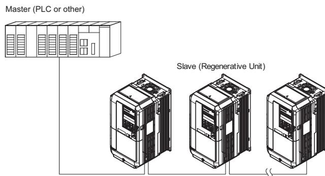
**Figure C.1 Connecting Multiple Regenerative Unit to a PLC**
