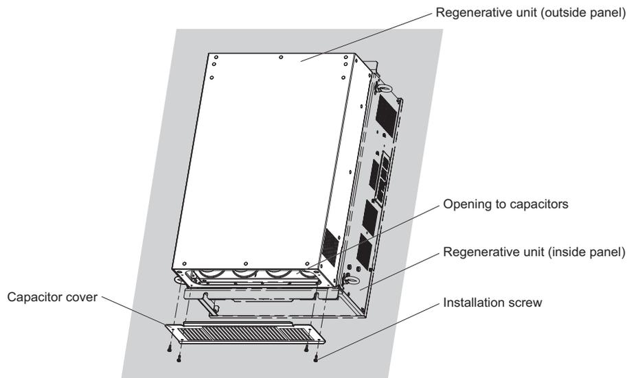
**Figure D.4 Capacitor Cover**
