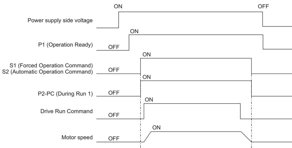
**Figure 4.3 Timing Chart for Power ON and Run Command Sequence**
