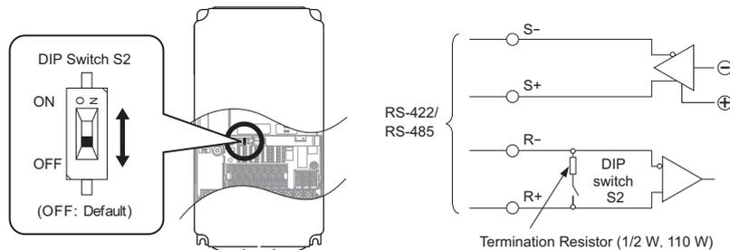
Figure C.3 Communication Terminals and DIP Switch S2
