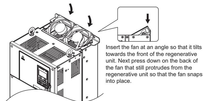
**Figure 6.10 Install the Cooling Fan: 2A0035, 4A0035, 4A0043**
