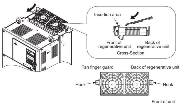
**Figure 6.11 Reattach the Fan Cover: 2A0035, 4A0035, 4A0043**
