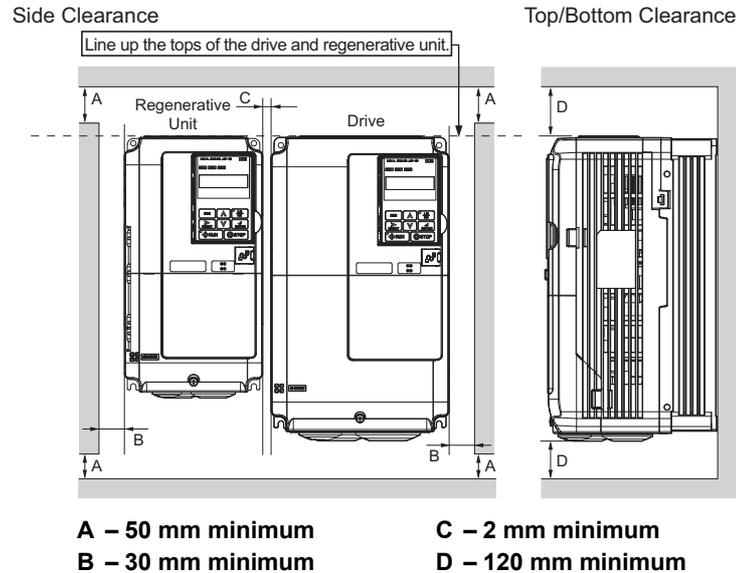
Figure 2.4 Space Between Regenerative Unit and Drive (Side-by-Side)
