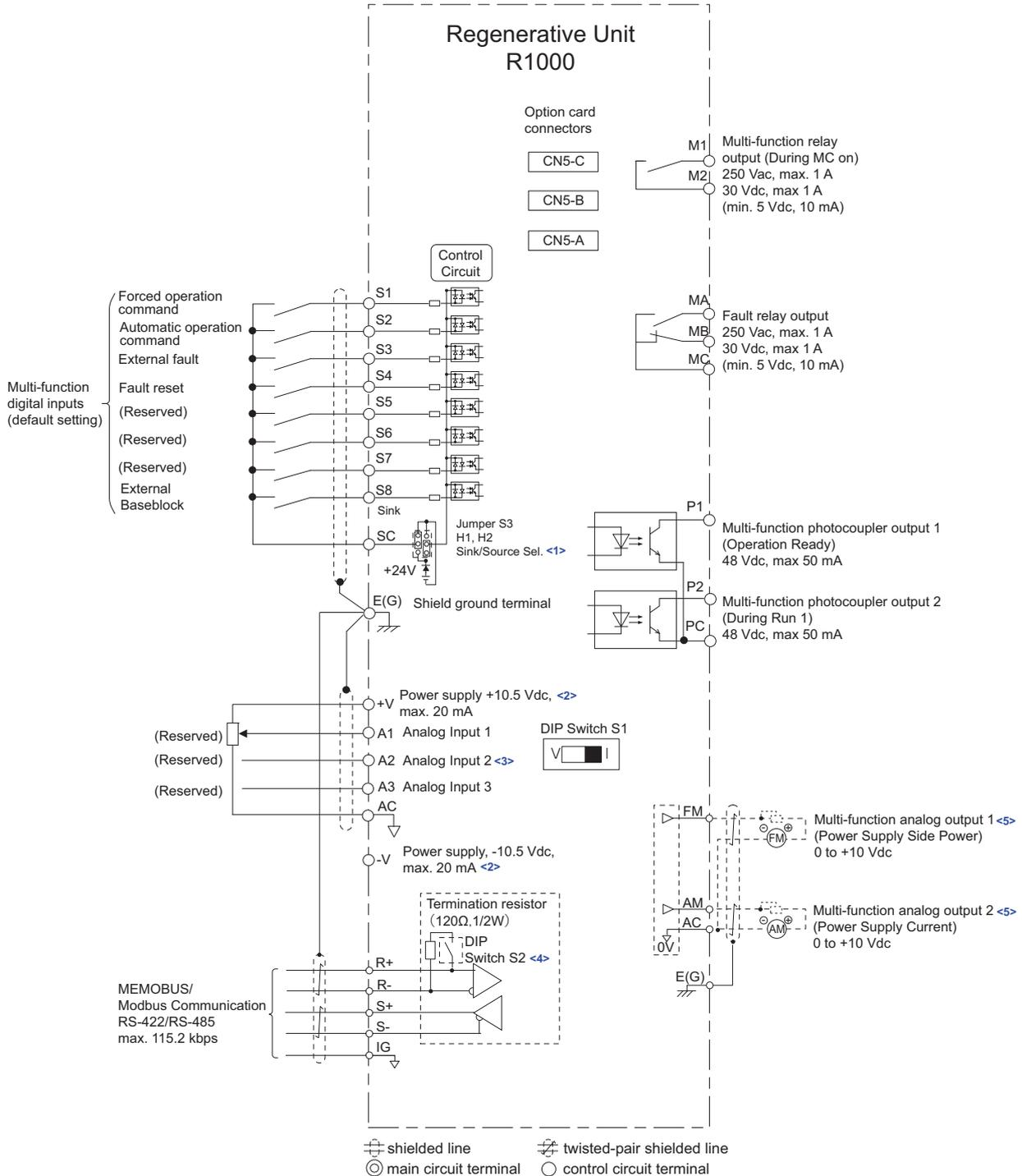
Figure 3.20 Control Circuit Wiring
