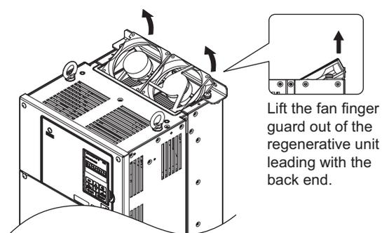
Figure 6.8 Remove the Cooling Fan: 2A0035, 4A0035, 4A0043
