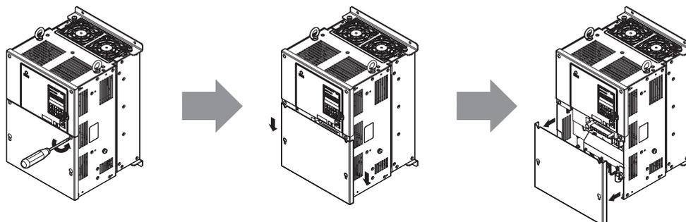
Figure 3.12 Removing the Terminal Cover on an IP00/Open Type enclosure Model
