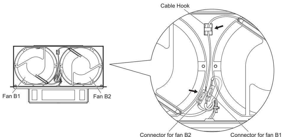
Figure 6.17 Cooling Fan Wiring: 2A0073, 4A0105, 4A0150
