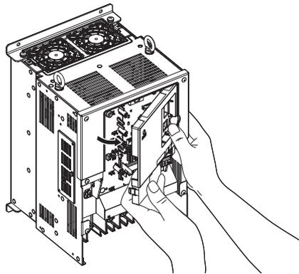
**Figure 3.17 Remove the Front Cover (2A0035 to 2A0105, and 4A0035 to 4A0300)****■ Reattaching the Front Cover****Models 2A03P5 to 2A0028, 4A03P5 to 4A0028**
