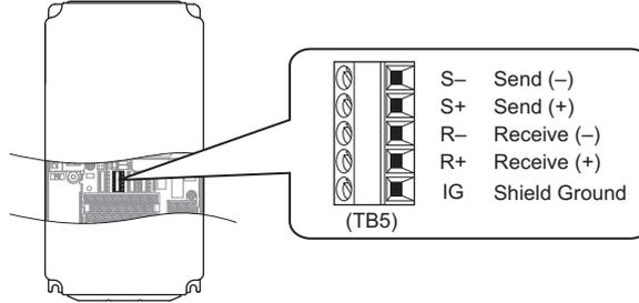
Figure C.2 Serial Communications Cable Connection Terminals (TB5)
