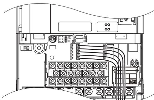
Figure 3.26 Terminal Board Wiring Guide
