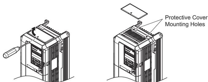
Figure 3.19 Removing and Reattaching the Top Protective Cover
