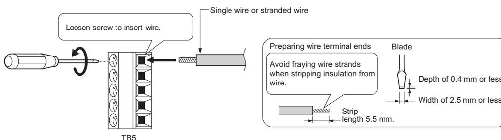
Figure 3.25 Terminal Block Wiring Guide
