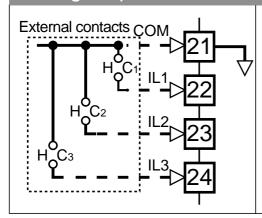
An impulsive (2 sec. at least) closing of contacts C1, C2, C3, permits the passage from AUTO/MAN, from Local/Remote Set point, recalling the 4 memorized Set points and launching of the programmed Set point. (see p. 16)
