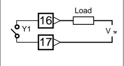
Universal and galvanically isolated. 2 relays are simultaneously present for discontinuous output with single or dual action (HEAT:COOL) and the signal for standard continuous output 4..20mA (or 0..10Vdc) which can also be Logic output 0/18Vdc).
