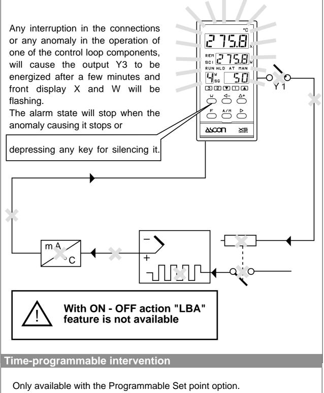
The ON or OFF state of the auxiliary outputs Y2 and/or Y3 can be selected for every segment of the programme. (See chapter 11)
