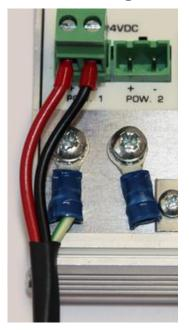
It is recommended to use a power supply with a ground lead (3-wire).
