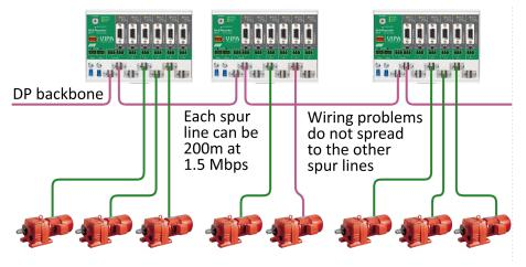
Long spur lines to instruments and the possibility to remove/insert them during operation. Short circuit protection on each spur line is automatically provided.
