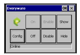
Note: The blue Everyware icon means that the terminal is offline. Press the "On" key to connect the terminal to the network (the icon turns green).
