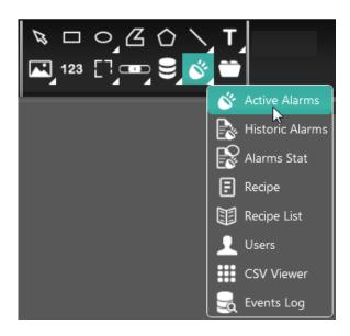
The "Active Alarms" icon on the "Graphics" menu is used to place an active alarms table on the page, drawing it with the mouse on the page.
