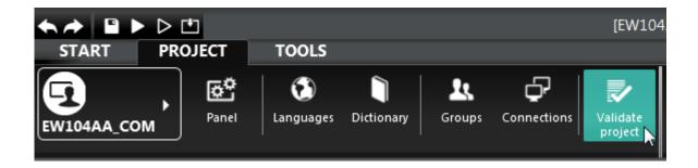
Validation is the operation that verifies the coherence of the objects entered in the project. The presence of any errors is reported in the following box.
