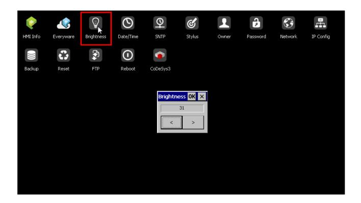
Use the relative keys to configure the brightness of the screen.
