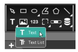
The "Text" (or "Label") icon in the "Graphics" menu is used to add text to a page, drawing the size of it on that page.
