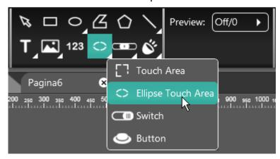
The "Sensitive area - Ellipse -" icon on the "Graphics" menu is used to add an elliptical sensitive area on the page, drawing it with the mouse on the page.
