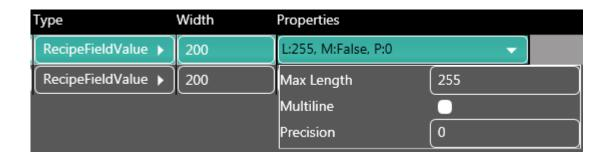
From the properties it is possible to define the maximum length of the recipe name (255 characters by default) and activate or deactivate the "Multiline" option, and establish the decimal precision of the recipe field, namely the number of digits after the decimal point.
