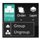
The "Grouping" function is used to group together two or more graphic elements so as to run cumulative operations on all of the objects at the same time.
