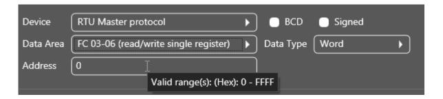
Note: The Binary-coded decimal (BCD) is a class of binary encodings of decimal numbers. In this format, each digit of a number is represented by a binary code of four bits, the value of which is between 0 (0000) and 9 (1001). For example, the number 127 is represented in BCD as 0001, 0010, 0111.
