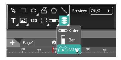
The "Indicator" icon on the "Graphics" menu is used to place an indicator on the page, drawing it with the mouse on the page.
