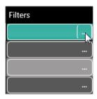
With the Filters option it is possible to enable Runtime display filters for the alarm log. For example, it is possible to associate a filter to the "AlarmOnTime" function to display only the alarms within a given period of time (chosen by the user).
