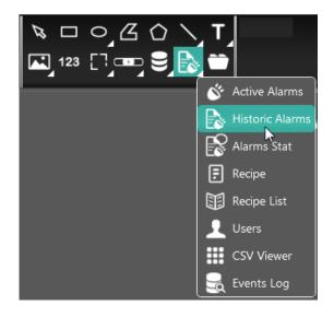
The "Alarm Log" icon on the "Graphics" menu is used to place an alarm log table on the page, drawing it with the mouse on the page.
