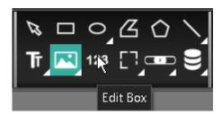
The "Edit Box" (or "Numerical field") icon in the "Graphics" menu is used to add an edit box to a page, drawing the size of it on that page.
