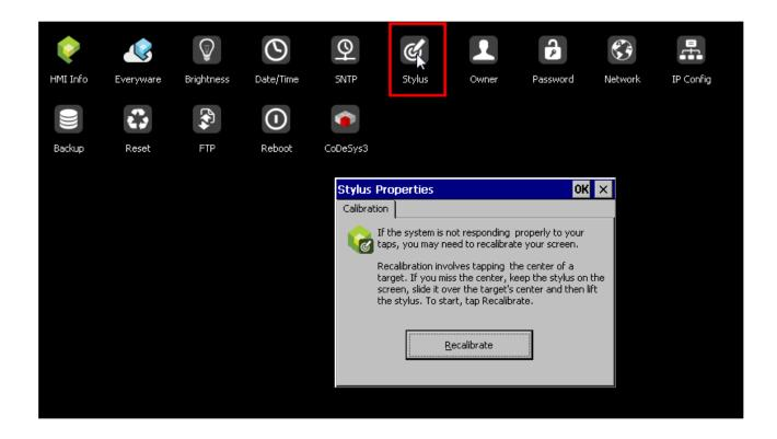
This is used to repeat, if necessary, the touch screen calibration procedure.
