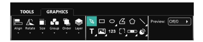
All of the graphic elements have been grouped together into three different sections of the menu. The first contains the following:
