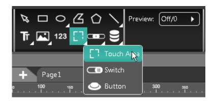
The "Sensitive area" icon on the "Graphics" menu is used to add a sensitive area on the page, drawing it with the mouse on the page.
