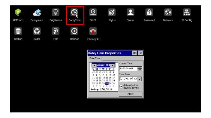
This changes date, hour and time zone. By enabling the "automatically adjust clock for daylight saving" check, the time automatically updates to BST or GMT.
