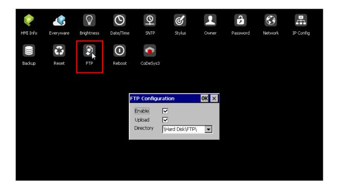
To enable the sharing service of a "FTP" (Files Transfer Protocol) folder.
