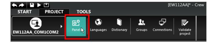
The "Panel" option shows a window where the user can view and enter the panel properties, such as: information, network, safety, system font behaviour and events.
