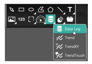
The "Data Log" icon on the "Graphics" menu is used to place a data log table on the page, drawing it with the mouse on the page.
