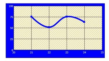
• HorLevels: the points on the graph are joined by a continuous curved line which flattens horizontally around the points.
