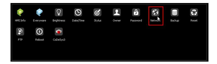
If the settings are correct, you will see the following image (Ethernet port 1 connected to the network correctly).
