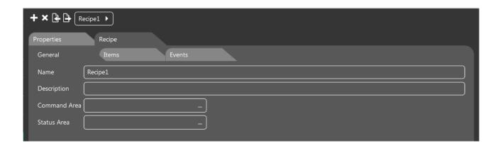
The "Command Area" and "Status Area" options offer the possibility of synchronising the recipe structure transfer through due reference tags (for more information refer to the "SyncMode - Synchronised transfer" section).
